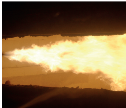
▲ By heating pure oxygen and fuel with fumes, combustion performance is increased by 50%.
