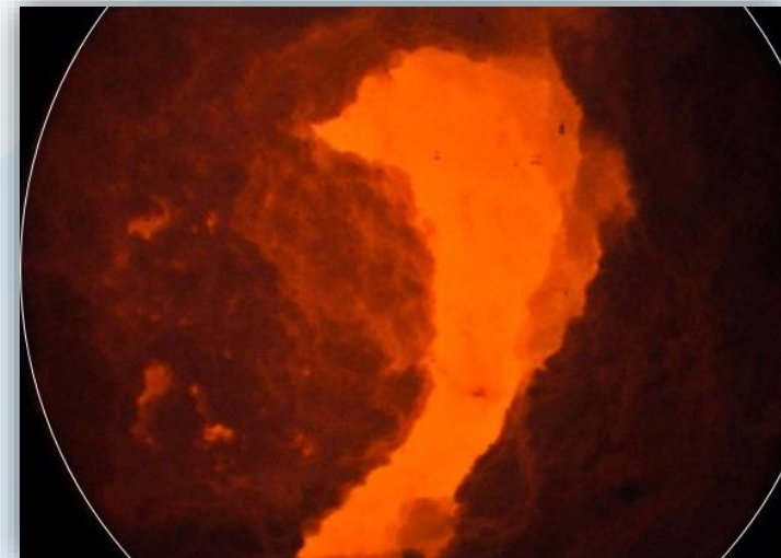
Clogging: \text{Na}_2\text{SO}_4 deposition (endoscopy image)
