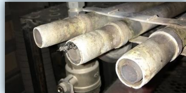
Carbon build-up on nozzle tip
